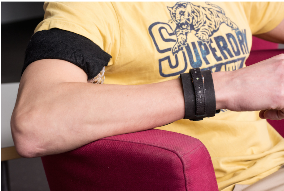
Figure 5.15: Male participant wearing the light bracelet during the study. On his upper arm he wears an additional armband that contains the controlling hardware, which is whipped with black felt for decorative reasons.
