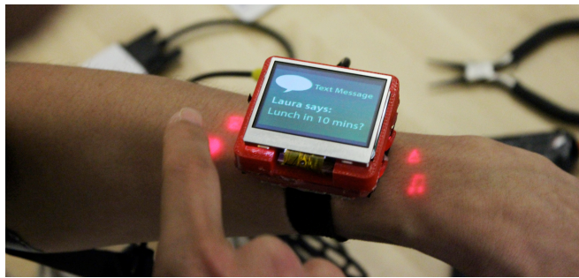
Figure 2.10: Skin Buttons : Tiny projectors integrated into a smartwatch project touch-sensitive icons on the user's skin [LXC + 14].
