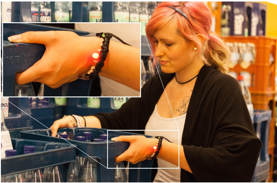
Figure 5.1: WaterJewel : Single light spots on a bracelet reflect the user’s daily fluid intake behaviour and thus help her to drink 2 litres in 8 evenly distributed servings over the day.
