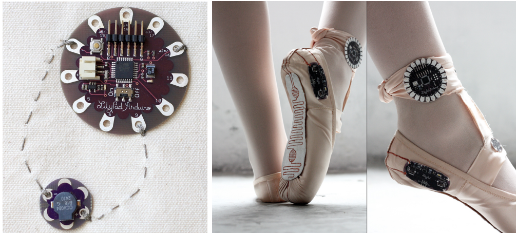
Figure 2.4: Left: Wearable electronics prototyping platform Arduino LilyPad. Right: E-Traces, a LilyPad project with a ballet shoe that captures dance movements and transforms them into visual sensations [Lil16].
