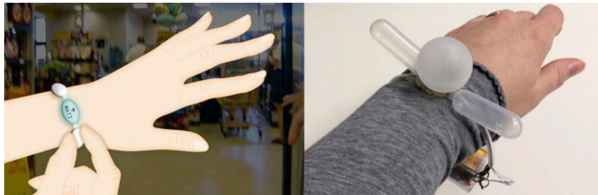
Figure 2.11: Squeezy Bracelet: Interaction concept (left) and prototype implementation (right) [PCH + 14].
