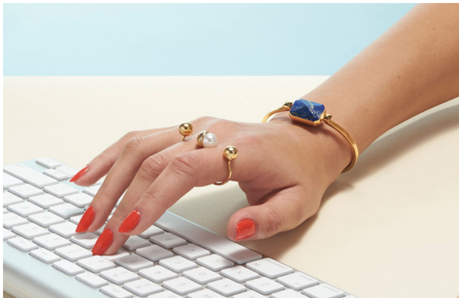
Figure 1.1: The Aries bracelet appears as jewellery and displays notifications from a smartphone via vibration patterns and a flashing light shining through a hole on the side of the bracelet. Image source: urbanwearables.technology
