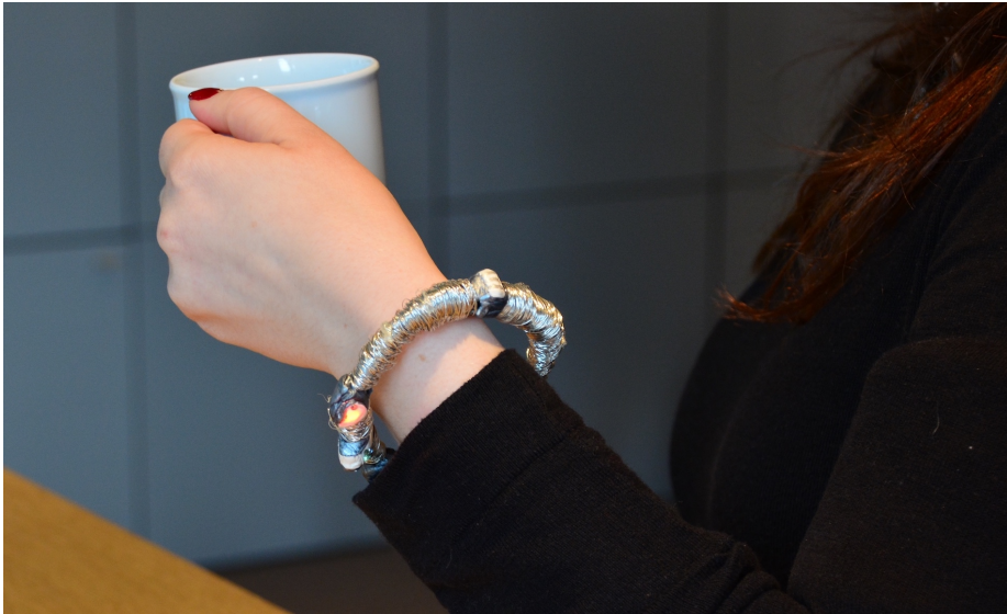
Figure 6.2: The TangibleApps bracelet consists of single elements - each offering a specific application - that are attached to a charm bracelet. Information is presented discreetly through light and vibration.
