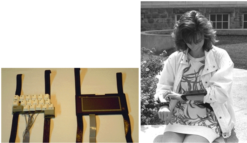
Figure 2.2: The first wrist-worn wearable computer consisted of a half, one-handed keyboard and a display, strapped to the user's forearms [MMB96].
