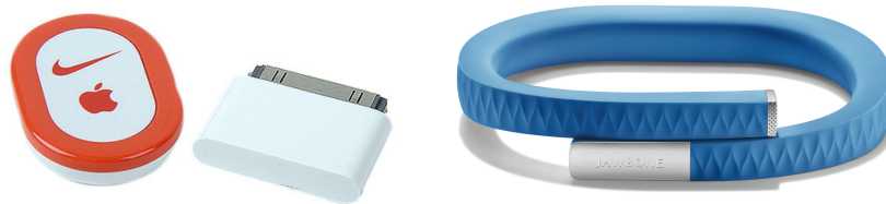
Figure 2.3: Left: The Nike+ iPod Sport Kit consists of a wireless transmitter put into a shoe (left) and a receiver plugged into an iPod music player (right) and offers the functionality of a pedometer; Right: Fitness and sleep tracker wristband Jawbone UP. Image sources: CNET, Taputapu Gadget Blog.
