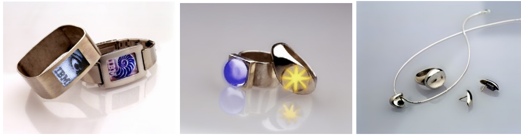
Figure 2.5: IBM Wearable Mobile Phone: a ring lighting up to notify of an incoming call (centre), a bracelet to display detailed information on the caller (left), as well as an earring and a necklace serving as speaker and microphone with another ring enabling TrackPoint input (right) [MCC01].
