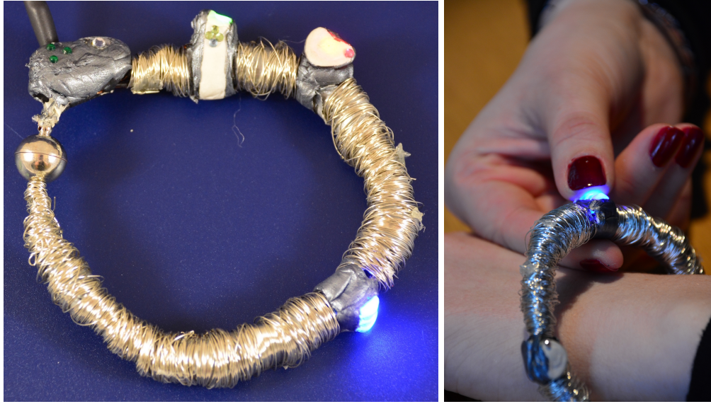
Figure 6.10: Left: Prototype of the TangibleApps bracelet. Elements are made up of modeling material that diffuses the light of underneath mounted LEDs. LEDs are glued on push buttons. Elements are kneaded into shapes and garnished with acrylic paint and appliqués. Silver wire is wrapped around copper wires to form the bracelet and enhance a jewellery look. Right: User pushes an element to make an input.
