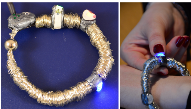
Figure 10. Left: Prototype of the Tangible Apps Bracelet . Elements are made up of modeling material that diffuses the light of underneath mounted LEDs. LEDs are glued on push buttons. Elements are kneaded into shapes and garnished with acrylic paint and appliques. Silver wire is wrapped around copper wires to form the bracelet and enhance a jewellery look. Right: User pushes an element to make an input.
