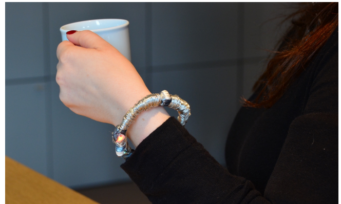
Figure 1. The Tangible Apps Bracelet consists of single elements - each offering a specific application - that are attached to a charm bracelet. Information is presented discreetly through light and vibration.
