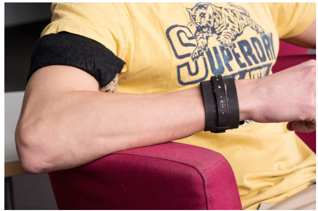
Figure 2: Male participant wearing the light bracelet during the study. On his upper arm he wears an additional armband that contains the controlling hardware, which is whipped with black felt for aesthetic reasons.
