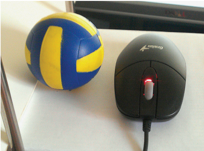
3 A ball and a mirror are used to measure the delay between user input and screen update.
