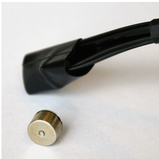
2 Close-up of the haptic actuator attached to the temples of the glasses.
