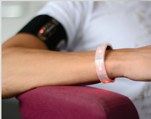
1 A participant wearing the prototype. The light bracelet is worn on the wrist and the armband with the electronics is attached to the upper arm.
