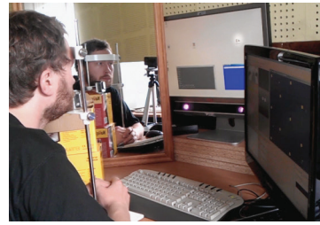
3 A ball and a mirror are used to measure the delay between user input and screen update.
