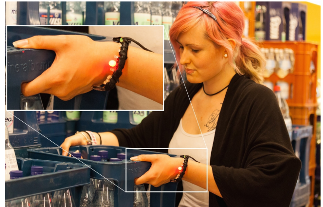
Figure 1. WaterJewel : Single light spots on a bracelet reflect the user's daily drinking behaviour and thus help her to drink 2 litres in 8 evenly distributed servings over the day.
