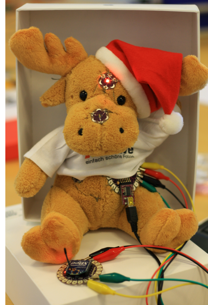
Figure 3: The Elch turns red when placed upside-down and green when shaken. Other sensors and actuators were used to make different sounds and vibrations depending on the interaction with the Elch.
